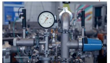
Leaks in the air distribution system can lead to significant energy losses. Testing for and repairing these leaks minimizes the unwanted loss of air pressure and increases the effectiveness of other optimization measures.
